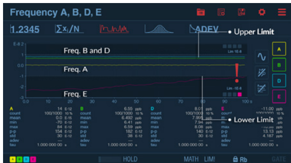
The time-line view reveals drift during the calibration
